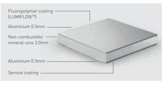
ALPOLIC<sup>TM</sup> A1 is manufactured from two 0.5mm thick aluminium cover sheets. These are applied to the non-combustible mineral core (3.0mm) in a special fusing process. The particularly durable fluoropolymer resin coating LUMIFLON $^{\text{TM}}$  is applied to one side of the cover sheets in a coil coating process using latest coil coating technology.
